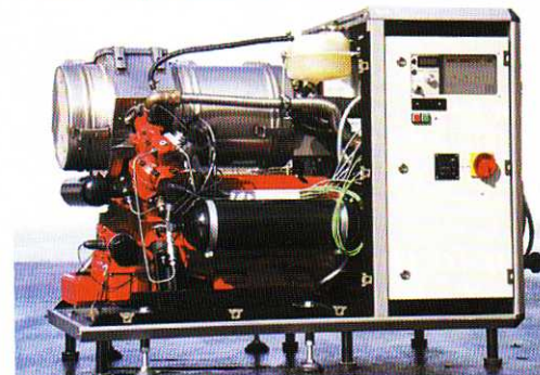
This 9 kW Stirling engine from the German company Dolo should be commercialized for wood pellet use in 2004
